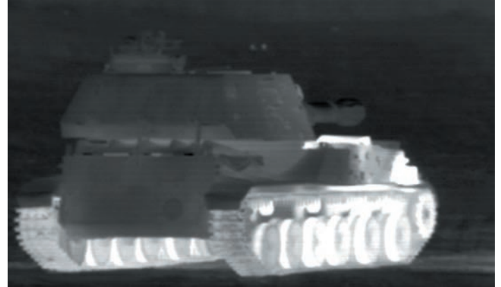
Example of a tank when viewed using an infrared camera
